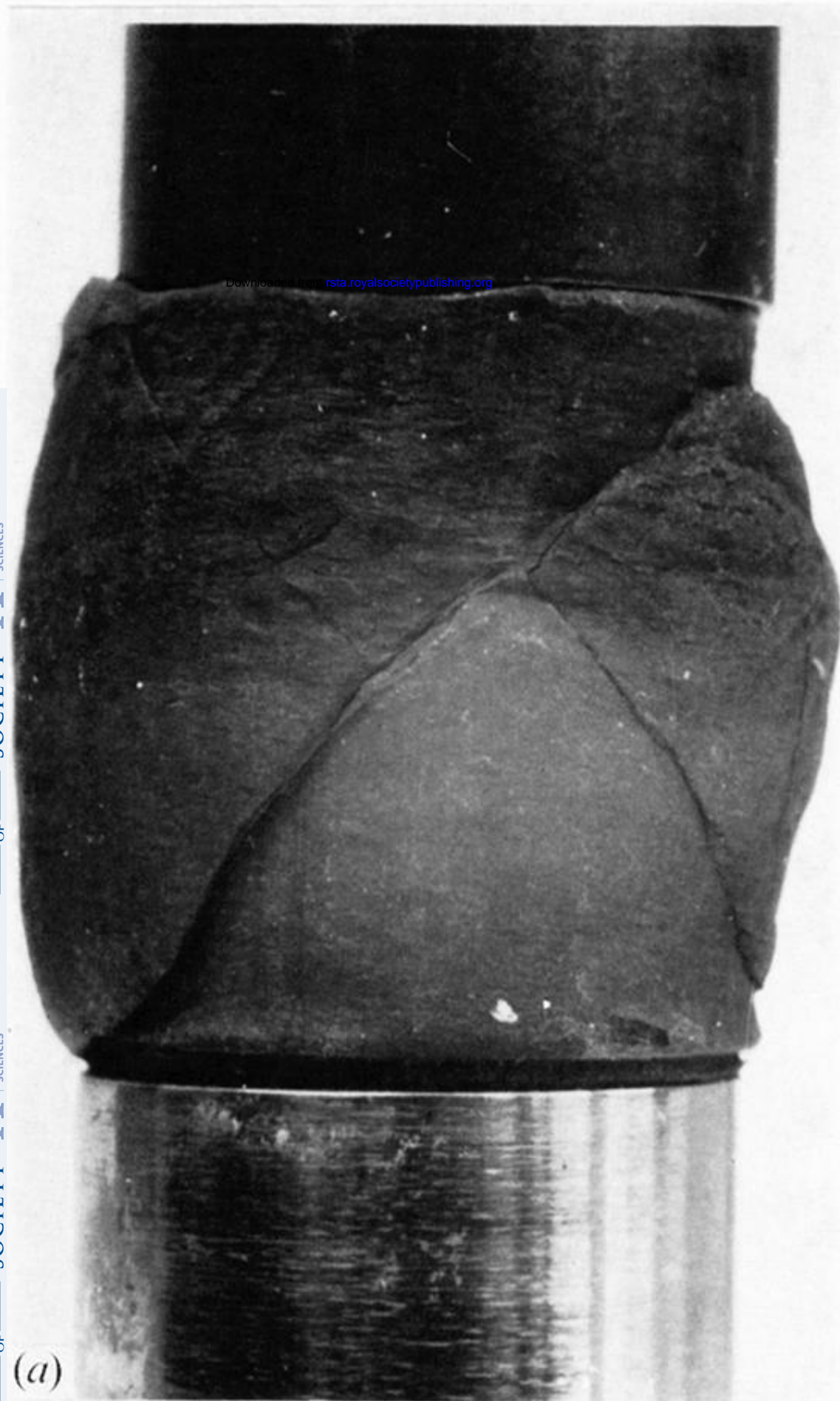
FIGURE 12. Samples consolidated at 62.1 \text{ MN m}^{-2} ( 9000 \text{ lbf in}^{-2} ) and tested (a) with cell pressure equal to consolidation pressure (test no. 19 B) and (b) unconfined (test no. 21 B). Surface texture shown in (c) for unconfined test.
