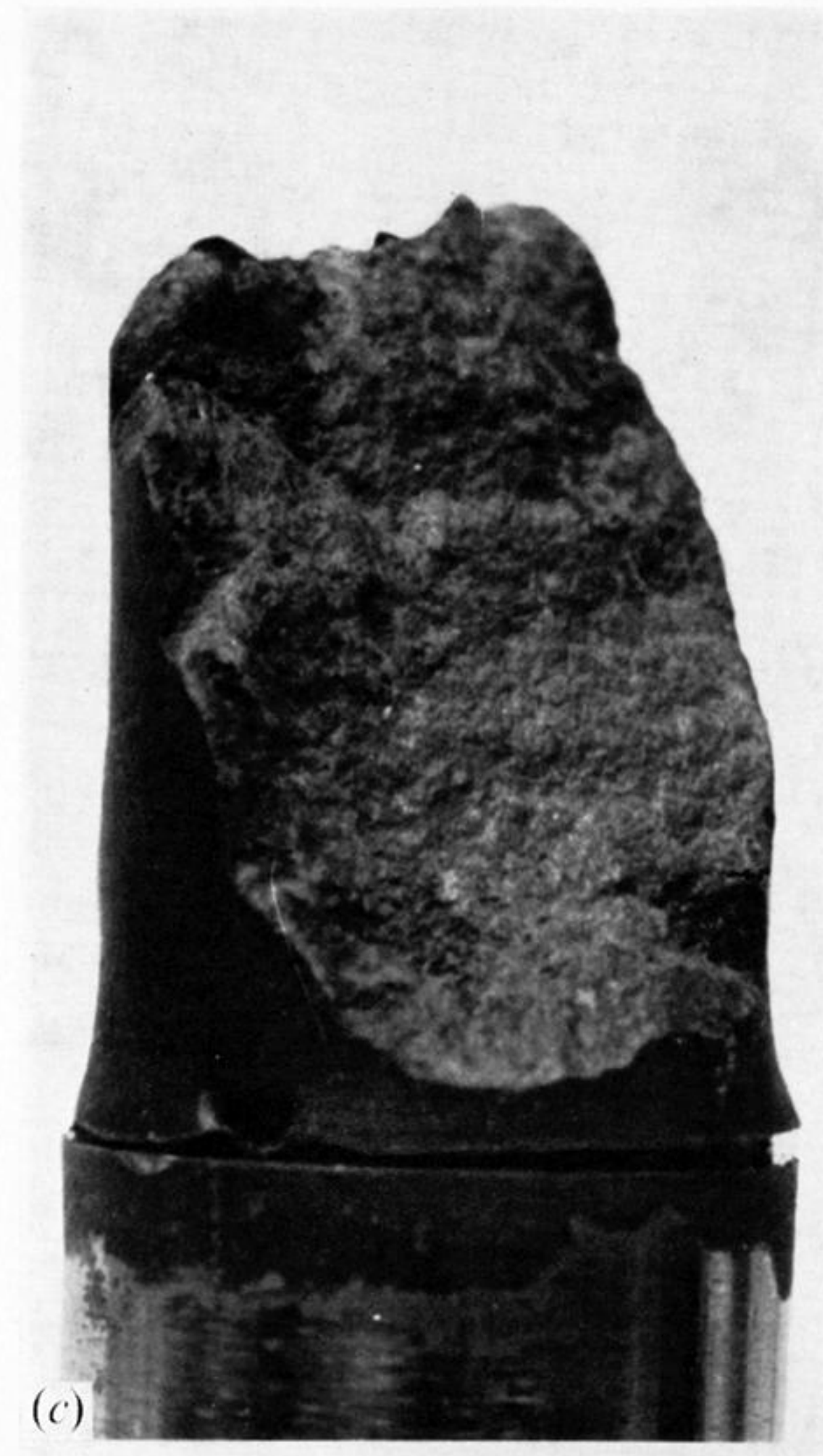
FIGURE 12. Samples consolidated at 62.1 \text{ MN m}^{-2} ( 9000 \text{ lbf in}^{-2} ) and tested (a) with cell pressure equal to consolidation pressure (test no. 19 B) and (b) unconfined (test no. 21 B). Surface texture shown in (c) for unconfined test.
