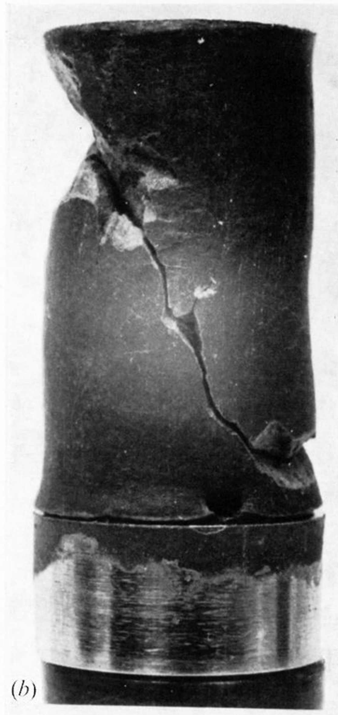
FIGURE 12. Samples consolidated at 62.1 \text{ MN m}^{-2} ( 9000 \text{ lbf in}^{-2} ) and tested (a) with cell pressure equal to consolidation pressure (test no. 19 B) and (b) unconfined (test no. 21 B). Surface texture shown in (c) for unconfined test.
